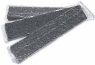
Rapid Roof Putty is a flexible, highly adhesive, fibre reinforced synthetic mortar. Rapid Roof Putty can be used with all types of concrete tiles and slates as an alternative to traditional concrete mortars, and provides weather tightness against driving rain and drifting snow.
