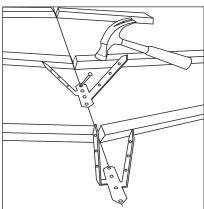
2. Secure a pair of hip batten straps to the hip rafter using the 3.35mm x 60mm stainless steel nails provided. At centres no greater than 550mm, fix the other straps up the length of the hip. Ensure that the first and last straps are fixed no more than 250mm from the fascia or hip/ridge intersections respectively.
