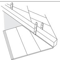
5. Lay the eaves course of tiles as normal with the eaves overhang equal on both sides of the hip and using a tile and a half neatly cut tiles to the line of the hip batten. The cut edge of the tiles should not be more than 30mm from the hip batten. Each cut tile must be twice nailed. If necessary drill an additional hole through the tile.
