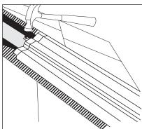
**8.** Cut one of the hip support trays between the eaves cut line indicated on support tray. Align the cut edge with the tail of the eaves course of tiles and secure the cut hip tile support to the hip batten with a clout nail placed through the top tab. Carry on clipping uncut hip tile support trays ensuring the tails of the trays are aligned to the line at the head of the fixed support. On reaching the ridge, mitre the support trays.
