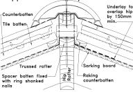
With rigid sarking, finish the board at the side of hip rafter. Fix a 50mm wide spacer batten to hip rafter with 100mm ring shank nails at 300mm centres. Top of spacer batten must be level with or not more than 12mm above top of counterbattens. Lap underlay 150mm over spacer batten. Fix raking counterbatten each side of spacer batten to support ends of tiling battens.
