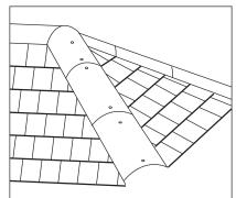
11. Fix the final ridge tile in position, ensuring the screw passes through the hole in the hip/ridge junction piece and the ridge tile traps the junction piece in place. Fix the final hip tiles in position. If necessary, adjust the height of the hip tiles with a screwdriver to give a true line.
