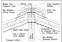
**1b.** When using a vapour permeable underlay the hip detail can be ventilated by placing a tiling batten between the Rollable Membrane and the Hip Tile Support Tray. See illustration above and table on inside flap of carton.
