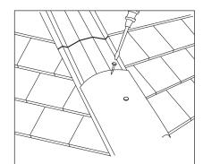
**9.** Place a purpose designed block end hip tile tight against the eaves tiles and secure with screws provided. Continue up the hip ensuring the hip tiles are butted together and that no individual hip tile is less than 300mm long.
