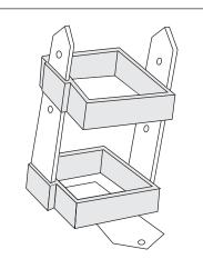
**3.** Place two spacer blocks onto each of the straps.
