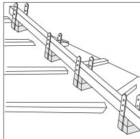
**4.** Place a timber batten (for size see table on inside flaps of carton) onto the blocks. Where it is necessary to use more than one length of batten, joints should be made over the supporting blocks. Do not fix the batten at this stage.
