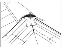
10. Where two hips meet a dry ridge, the intersection should be weathered using the hip/ridge junction piece (supplied separately). The three mitred tiles must be cut from full length tiles using the template provided. Re-drill the cut hip and ridge tiles to provide two fixings per tile. (Other forms of junction may be weathered using the flexible membrane as a saddle. Lead or Rapid Flashing will also provide a suitable alternative.)
