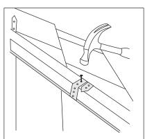
**6.** Secure the hip batten in position by wrapping the stainless steel straps around the batten and fix with the 2.65 x 30mm stainless steel clout nails provided.
