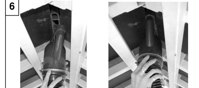
Connect the Terminal Adaptor to the Terminal ensuring the four lugs on the Terminal engage into the four holes in the Terminal Adaptor. Apply downward pressure on the Terminal to ensure a satisfactory connection. The free end of the Flexible Pipe is then connected to the main stack of the soil venting pipe or mechanical extraction pipe.
