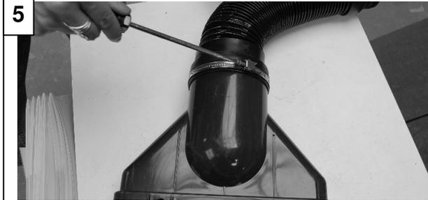
For soil venting or mechanical extraction, fix the Flexible Pipe onto the Terminal Adaptor by tightening the clip with a screwdriver to provide an airtight joint. Ensure the worm drive section of the clip is placed on the overlapped neoprene cuff area.
