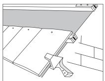
**5.** Set all tile courses 5mm back from the batten end on each verge. Ensure that the eaves tile is fully inserted into the Eaves Closure Unit. The interlocks of left hand verge tiles must be removed.
