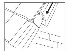
**9a.** Offer up the next unit as normal and tip it onto its outside face. Engage the bottom of the verge unit behind the installed one and slide it downwards to require position.
