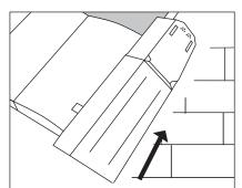
7. Clip the first Ambi-Dry Verge Unit over the Eaves Closure Unit. Slide the Ambi-Dry Verge Unit in the direction of the ridge until the tail coincides with the tail of the tile.
