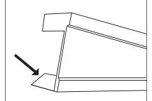
**6.** Depending on the hand of the verge, prepare the Ambi-Dry Verge Units by snapping out the relevant section. Picture above shows a right hand Ambi-Dry Verge Unit being prepared.
