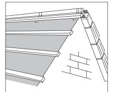
1. Felt and batten the roof, carrying the underlay over the full width of the gable and extending the tiling battens beyond brickwork, bargeboard or gable ladder by 45mm. Ensure all battens project by the same distance to achieve a straight verge line.
