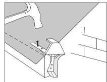
4. Using the nails and clip provided in the Eaves/Ridge Pack, fix the Eaves Closure Unit to the fascia as shown. At this stage one of two approaches may be adopted:
