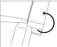
**9b.** Once in position, tip/turn the unit upright to the normal position engaging the lugs that lock the units in place. Slide the unit upwards to line up with the adjacent tile, ensuring lugs are engaged. Fix through batten end clip.
