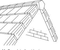
**11.** Complete the ridge/verge junction with a Block-end Ridge Tile.
