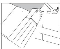
**8.** Ensuring contact with the head of a tile, nail the Ambi-Dry Verge Unit into the Batten End Clip. Nail through the most convenient hole using the 65 x 3.35mm nail provided.
