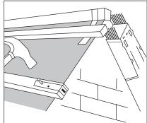
2. Using the 20 x 2.65mm dia. nails provided, fix a Batten End Clip to each tiling batten.
