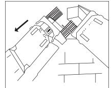
**10.** Mesh the Ridge Comb Units together before clipping onto the top two Ambi-Dry Verge Units. This will prevent bird access.
