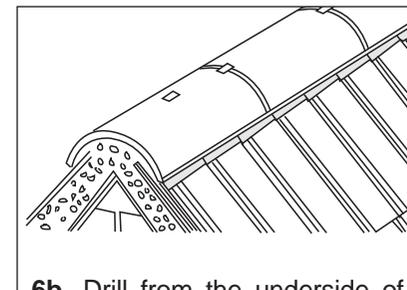
6b. Drill from the underside of the ridge tile a 6mm dia hole in the dead centre. Install the end of the ridge tile onto the verge mortar bedding using the screw, washer and plate provided, screw using a Pozidrive no 3 screw bit until the washer will not turn between the fingers. Flush off the mortar bedding in the usual manner. The remaining ridge tiles should be installed as per illustration 5c.
