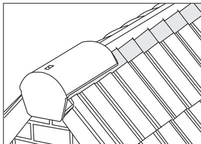
5b. The block-end ridge tile should be installed tight against the dry verge system whilst ensuring that the fixing screw lines up with the centreline of the ridge batten. Using the screw, washer and plate provided, use a Pozidrive no 3 screw bit and tighten the washer until it will not turn between the fingers.
