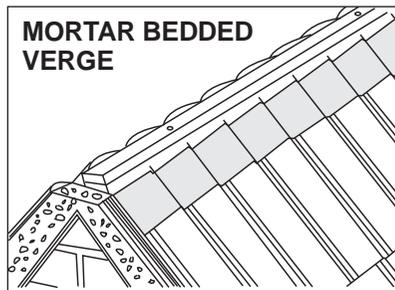
6a. With a mortar bedded ridge end, the batten should be cut 100mm back from the flush face of the mortar. The Rollable Membrane should be cut 50mm back from the face of the mortar.
