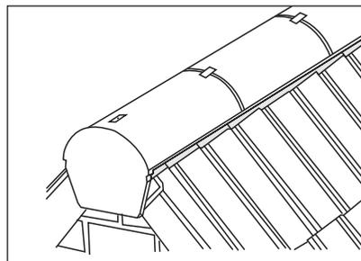
5c. Place a ridge to ridge seal and plate between each pair of adjacent ridge tiles. Ensure that the ridge tiles are butted up tight to the seal with the plate on top of the ridge tiles and that the ridge tiles line up with the centreline of the ridge batten. Screw the pre-installed ridge fixing screw into the centre of the ridge batten, until the washer will not turn between the fingers.
