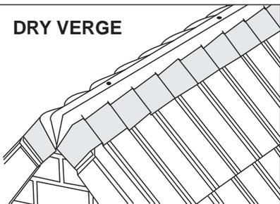
5a. The ridge batten should be finished inline with the end of the tiling battens. The Rollable Membrane should be neatly rolled down the vertical face of the dry verge and tucked back under the verge system.
