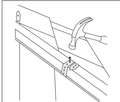
6. Secure the hip batten in position by wrapping the stainless steel straps around the batten and fix with the 2.65 x 30mm stainless steel clout nails provided.
