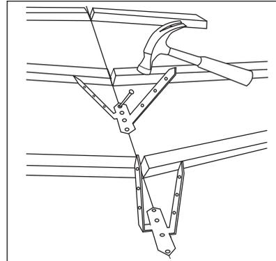
2. Secure a pair of hip batten straps to the hip rafter using the 3.35mm x 60mm stainless steel nails provided. At centres no greater than 550mm, fix the other straps up the length of the hip. Ensure that the first and last straps are fixed no more than 250mm from the fascia or hip/ridge intersections respectively.
