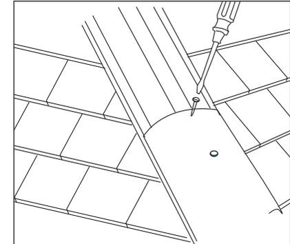
9. Place a purpose designed block end hip tile tight against the eaves tiles and secure with screws provided. Continue up the hip ensuring the hip tiles are butted together and that no individual hip tile is less than 300mm long.
