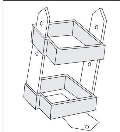
3. Place two spacer blocks onto each of the straps.
