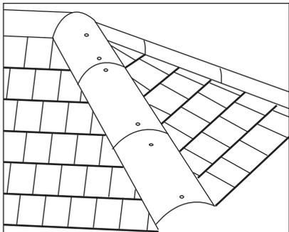
**11.** Fix the final ridge tile in position, ensuring the screw passes through the hole in the hip/ridge junction piece and the ridge tile traps the junction piece in place. Fix the final hip tiles in position. If necessary, adjust the height of the hip tiles with a screwdriver to give a true line.
