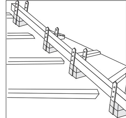
4. Place a 50mm wide batten onto the blocks. Use a batten height of 38mm for pitches up to 50° or 25mm for pitches above 50°. Where it is necessary to use more than one length of batten, joints should be made over the supporting blocks. Do not fix the batten at this stage.
