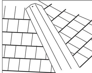
8. Cut hip tray to suit at the eaves and secure to the hip batten with a single clout nail at its centre point to hold it in place. Where more than one tray is required to complete the hip, overlap on top of the one already fixed by 200mm. Where two hips meet at the ridge, mitre the hip trays together.
