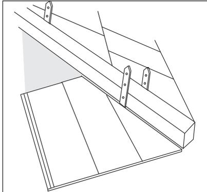
5. Lay the eaves course of tiles as normal with the eaves overhang equal on both sides of the hip and using a tile and a half neatly cut tiles to the line of the hip batten. The cut edge of the tiles should not be more than 30mm from the hip batten. Each cut tile must be twice nailed. If necessary drill an additional hole through the tile.
