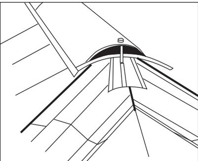
**10.** Where two hips meet a dry ridge, the intersection should be weathered using the hip/ridge junction piece (supplied separately). The three mitred tiles must be cut from full length tiles using the template provided. Re-drill the cut hip and ridge tiles to provide two fixings per tile. (Other forms of junction may be weathered using the flexible membrane as a saddle. Lead or Rapid Flashing will also provide a suitable alternative.)
