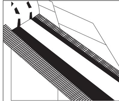
7. Starting from the eaves, dress the Rollable Membrane centrally over the hip batten ensuring all gaps at the eaves are covered. Remove backing strip from the adhesive section and neatly dress onto the tiles. Adhesion will be improved if the tiles are clean and dry. Continue up the full length of the hip, overlapping each roll by at least 50mm. Continue up and over the ridge batten.
