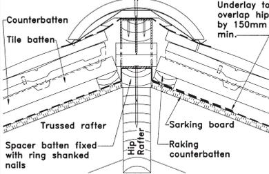
With rigid sarking, finish the board at the side of hip rafter. Fix a 50mm wide spacer batten to hip rafter with 100mm ring shank nails at 300mm centres. Top of spacer batten must be level with or not more than 12mm above top of counterbatens. Lap underlay 150mm over spacer batten. Fix raking counterbatens each side of spacer batten to support ends of tiling battens.
