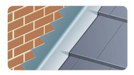
Rapid Flashing can be used instead of lead on the majority of pitched roof apllications. The unrivalled speed and ease of installation enables standard flashing details to be completed up to twice as quickly as with lead, offering a viable and safer alternative to traditional methods.
