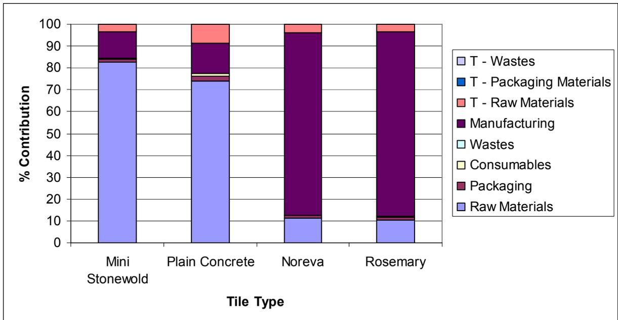
**Figure 4: Breakdown of Contributions to the Embodied Carbon Footprint<sup>5</sup>**
