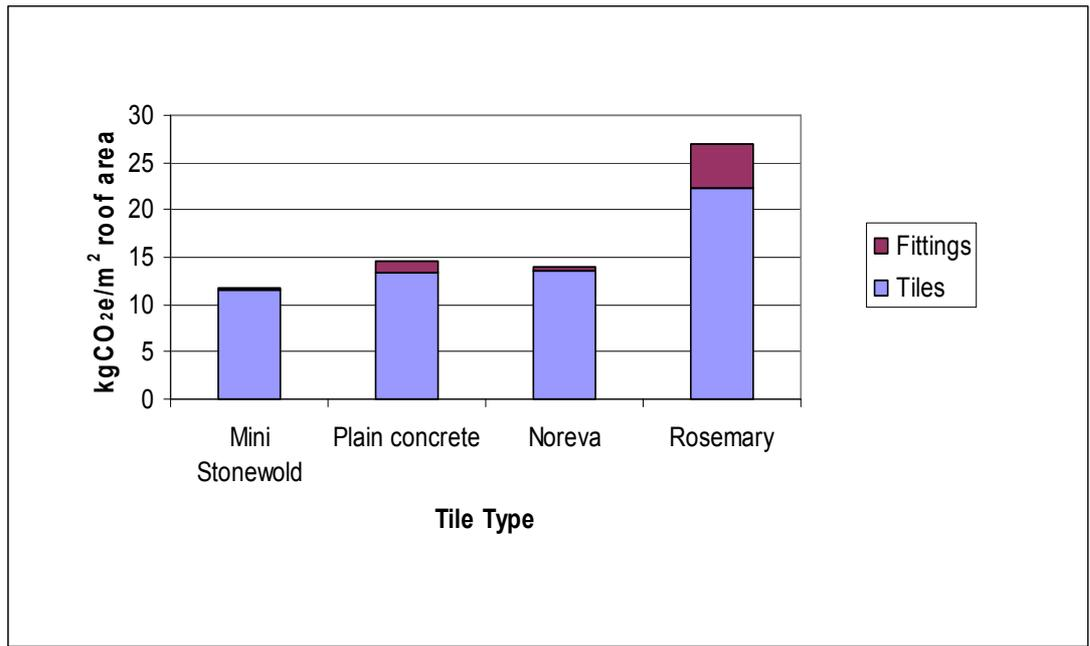
**Figure 1: Embodied Carbon Emissions per m<sup>2</sup> Roof Area for a 2 Bedroom Terraced New Build House**
