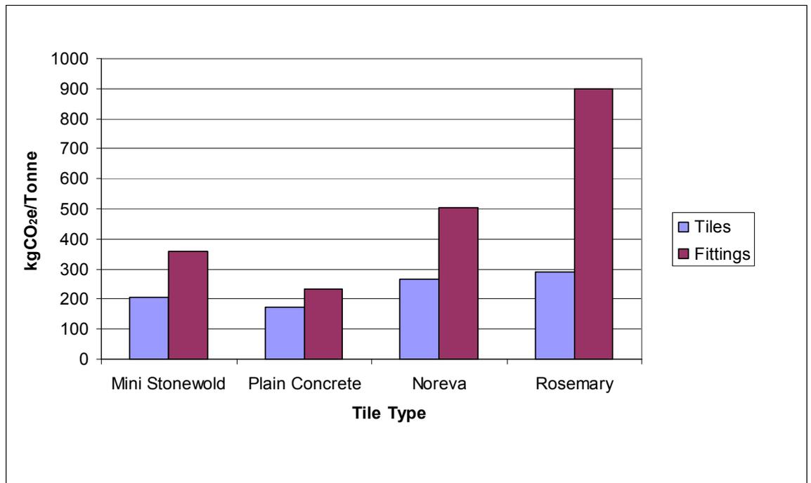
**Figure 3: Embodied Carbon Emissions comparison between Tiles and Fittings**
