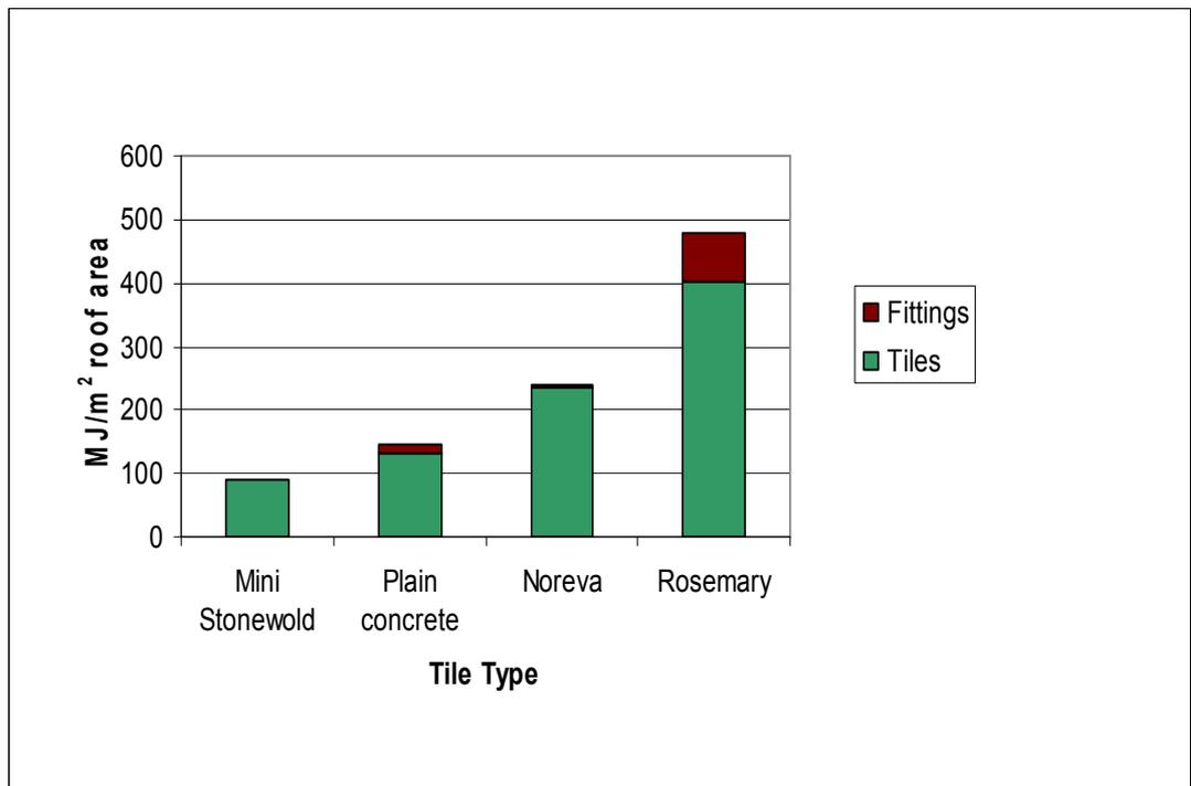
**Figure 2: Embodied Energy per m<sup>2</sup> Roof Area for a 2 Bedroom Terraced New Build House**
